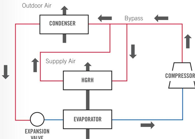
(Fig. 3) Simplified Hot Gas Reheat Schematic
