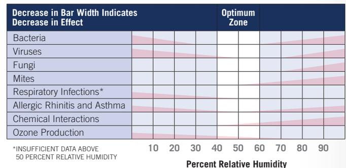
(Fig. 2) Humidity Ranges via Criteria for Human Exposure to Humidity in Occupied Buildings<sup>1</sup>
