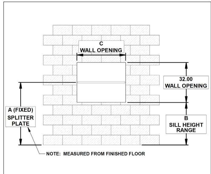
Split No Exhaust Wall Sleeve and Louver Dimensions and Mounting
