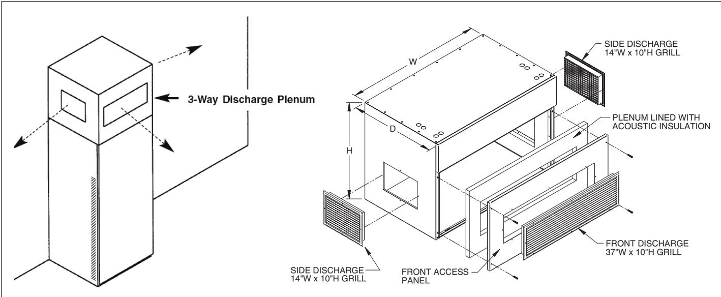
Figure 8.2 - Top Discharge Plenum
