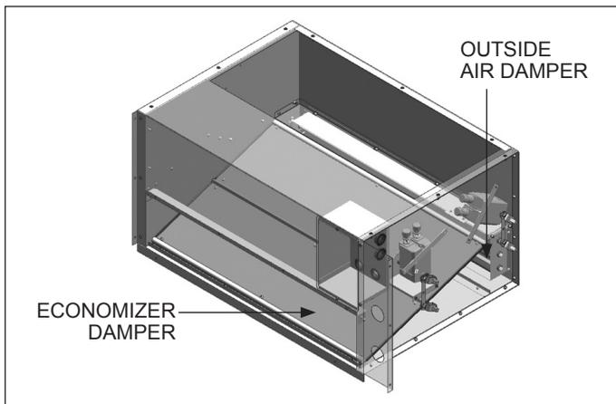
**C, H = Exhaust Recovery Ventilation (ERV) with Outside Air Damper**
