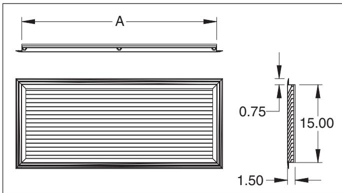
Figure 23.4 - Standard Wall Opening
