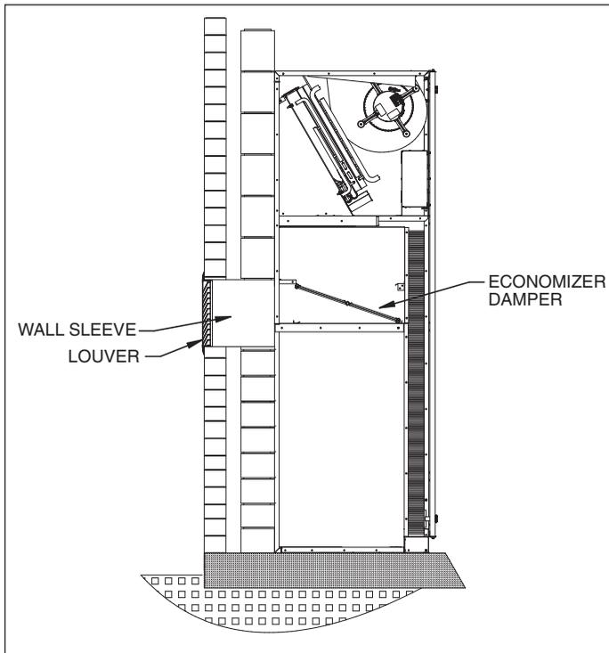
Figure 23.3 - Standard Wall Sleeve
