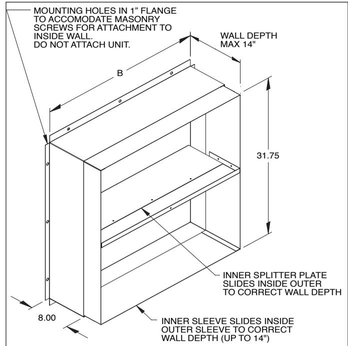
Figure 22.4 - Standard Single Wall Opening
