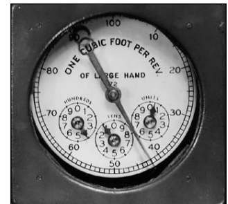
Figure 9 Dials of Typical Gas Meter
