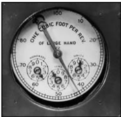
Figure 10 Dials of Typical Gas Meter
