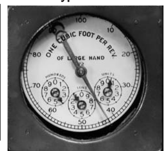
Figure 10 Dials of Typical Gas Meter
