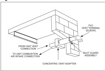
Figure 11.2 - Vertical Concentric Vent Kit
