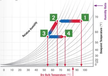
(Fig. 1) Dehumidification Process on Psychometric Chart
