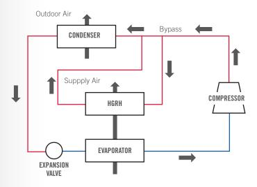
(Fig. 3) Simplified Hot Gas Reheat Schematic
